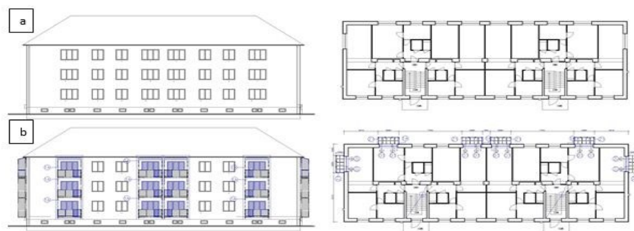
Fig. 1: Floor plans and views of the analysed residential building, a - original condition, b - proposed condition
